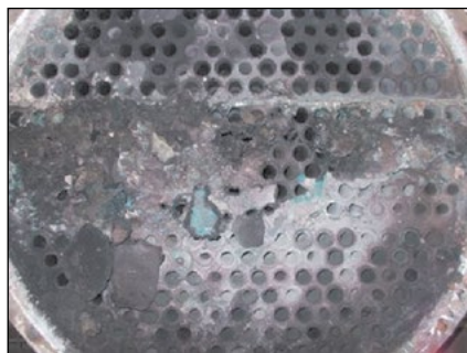
Fig. 2: Fouling as experienced in evaporator of effluent from dyestuff producer
